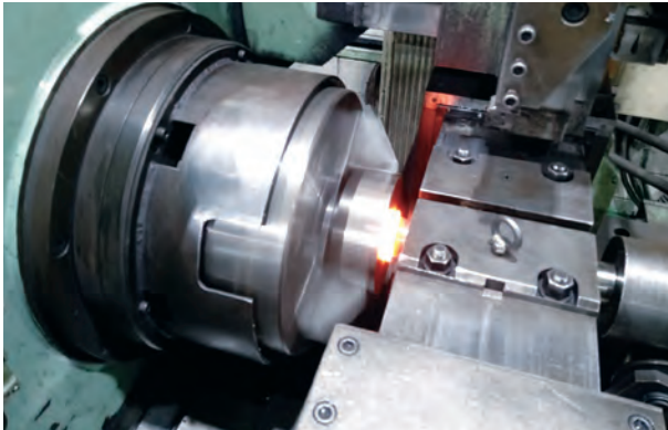
Condition of friction welding joint
