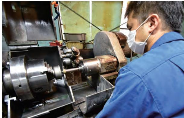
Picture of processing by internal grinder
