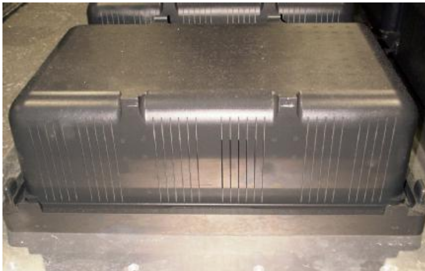
“Multi-Merit die” placed linear slit on molding surface (Core type on the photo)
